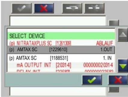
3. Press the required sensor for the RTC module and confirm by pressing **ENTER** below the selection list.
