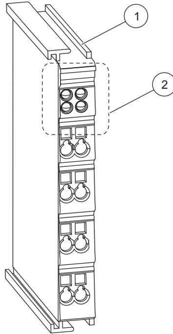
1 Analog or digital input or output module or bus termination module
