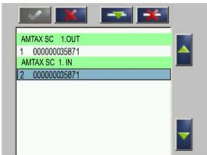
6. To sort the sensors in the order specified for the RTC module, press the sensor and use the arrow keys to move it (Figure 4, item 5).
