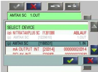
5. Select the second sensor for the RTC module and confirm by pressing **ENTER** below the selection list.
